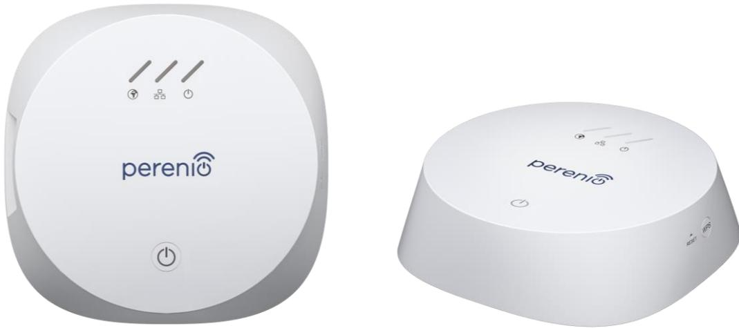
**Figure 1 - The PEACG01 Control Gateway Exterior**
